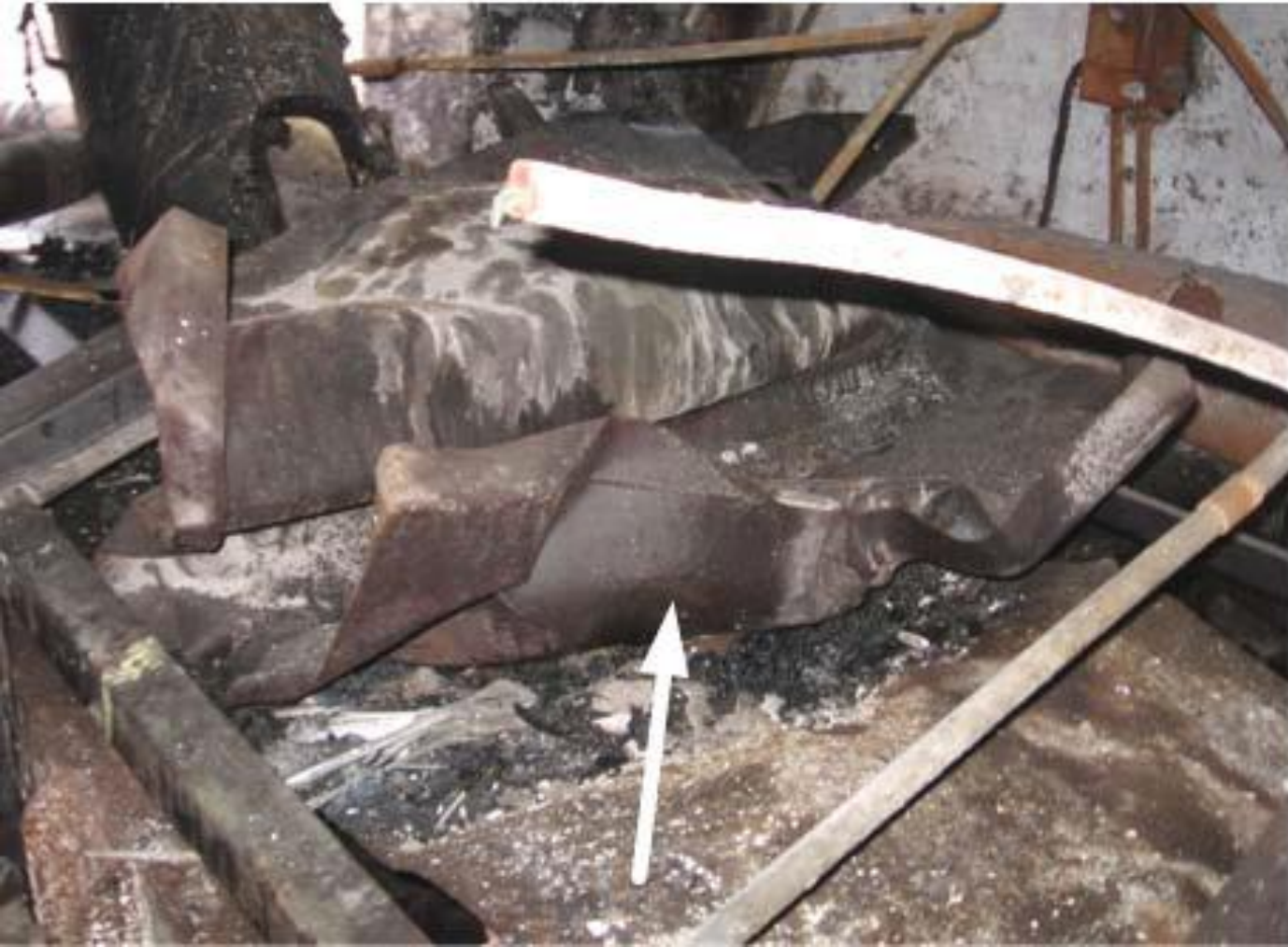
Steel belt covers (arrows) crumpled from an initial dust explosion inside the steel belt enclosure (steel frame structure, right photo)
