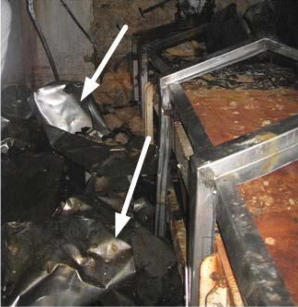
Steel belt covers (arrows) crumpled from an initial dust explosion inside the steel belt enclosure (steel frame structure, right photo)
