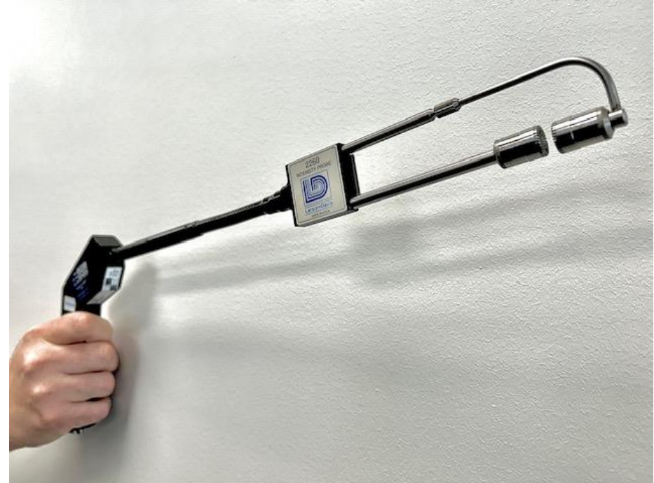
Method 2: "Scan" over the source with a sound intensity probe (ISO 9614)
